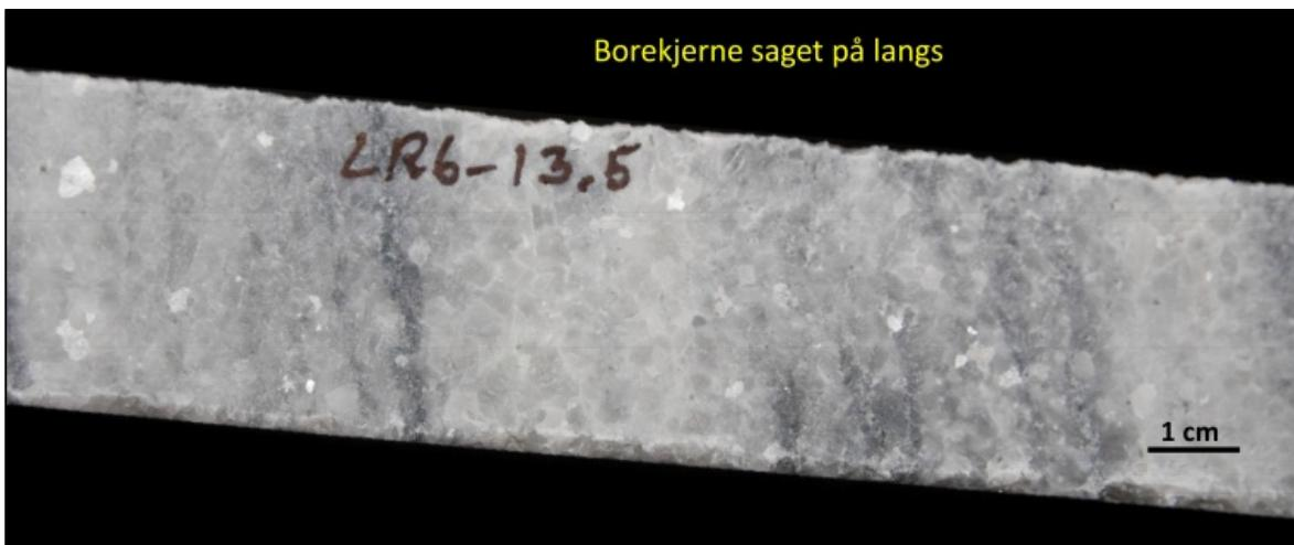
Fig. 6: Photograph of drill core of coarse-grained calcite marble.
